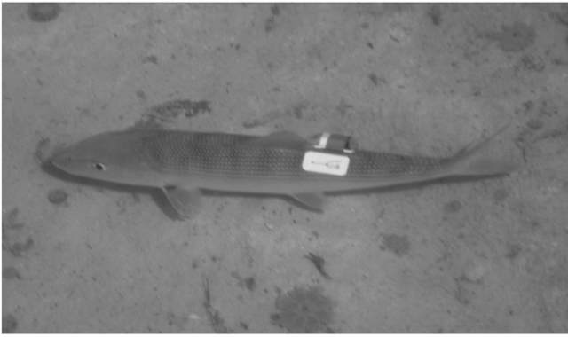
Fig. 1. Location of accelerometer attachment on bonefish for quantifying behavior after simulated angling stress.
