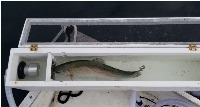
FIGURE 1. Rainbow Trout held in the flow box. Fish were positioned facing the direction of the flow, and the lid was closed during the treatment.
